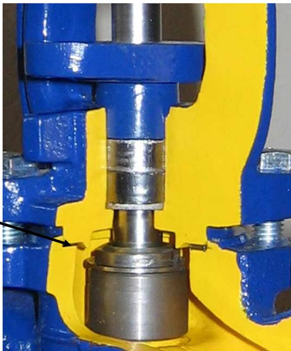
Everytime when valve bonnet was disassembled sealing surface should be cleaned. During assembly it should be applied new gasket of the same type as previously used. Body-bonnet bolt connections should be tighten when the valve is at open position. The bolts should be tighten evenly and crosswise by torque wrench.
