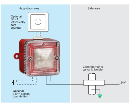
The BA386 is an intrinsically safe field mounting beacon which produces a bright flashing warning signal in a hazardous area. This beacon is significantly less expensive than the traditional Xenon devices, although it has a similar light output, flashes more frequently and is available in five different colours.
