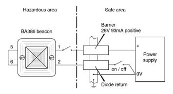
Fig 5 Single stage alarm using two channel barrier.
