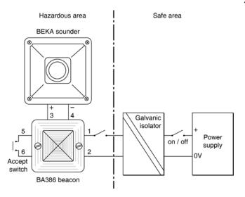
Fig 8 Combined beacon and sounder with alarm accept switch
