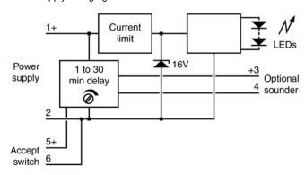
Fig 1 Simplified block diagram
