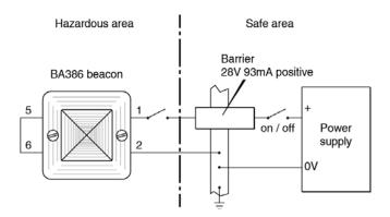
Fig 4 Using a single channel barrier.
