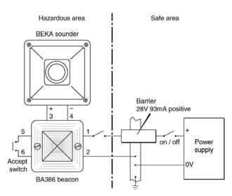
Fig 6 Combined beacon and sounder with alarm accept switch
