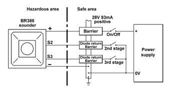
Fig 6 Multi-stage alarm using Zener barriers.
