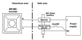
Fig 5 Single stage alarm using two channel barrier.
