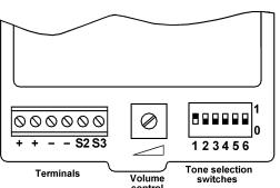
Fig 3 Location of field terminals and controls.
