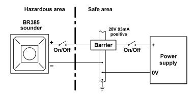
Fig 4 Single stage alarm using single channel barrier.
