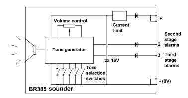
Fig 1 Simplified block diagram
