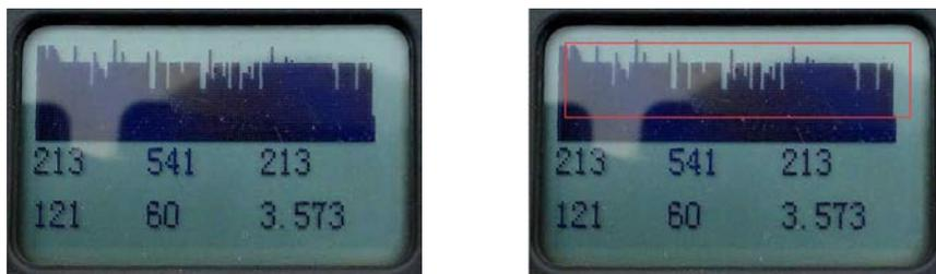
Fig. 10 Echo Pattern under Strong Interference
