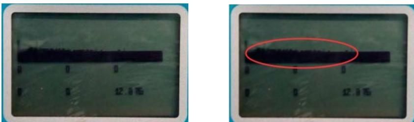
Fig. 6 Echo Pattern under Electromagnetic Interference
