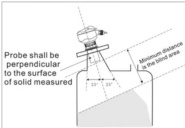
Extended connecting pipe for solid medium measurement
