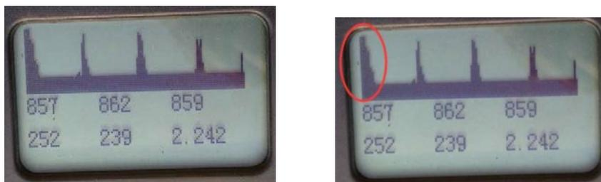
Fig. 2 Echo Signals after Resonance Problem Solved
