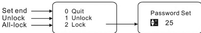
★ If the parameters are locked, press SET and enter in the unlocking interface for parameter locking:
