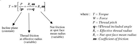
In simplified form, for lubricated fasteners, washers, nuts etc (see also Section 6.4), the relationship between torque and fastener load may be represented as:
