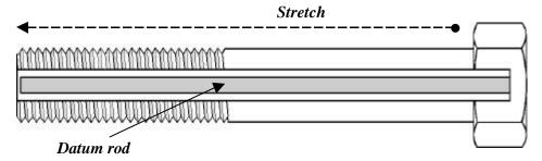
Measurement of bolt stretch using a micrometer is time consuming and may not provide control of preload with sufficient accuracy. The use of ultrasonics overcomes many of the disadvantages, offering a more accurate method for the determination of bolt stretch<sup>5</sup>, although not always very convenient and requires a high degree of operator skill. Fastener stretch can also be monitored by using tension control fasteners, which are pre-set to the required load.
