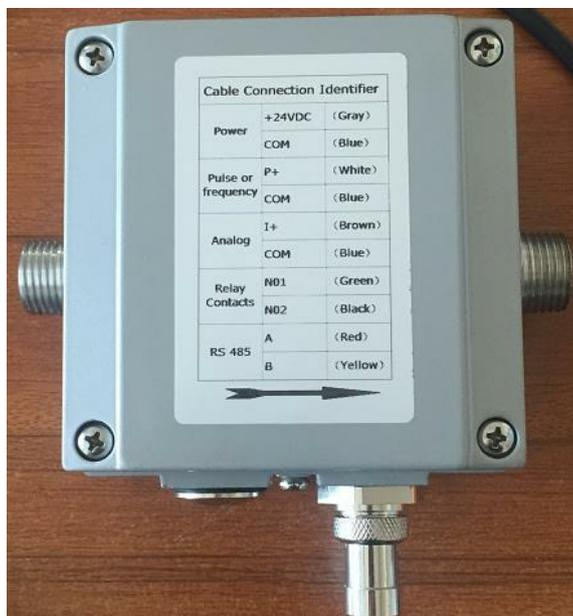
Fig. 5.1 Cable Connection Identifier
